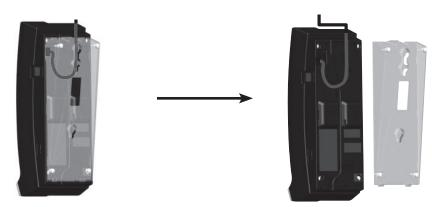
3. Turn the mounting bracket upside down. Remove the telephone line cord from the wire duct and then route it through the groove on the bottom part of the mounting bracket. Insert the small tabs on the mounting bracket into the upper slots on the telephone base. Then press the large tab on the mounting bracket and firmly push it into the lower groove on the telephone base.
