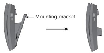
4. Plug the Cat-5 network cable back into the network wall jack with Power over Ethernet (PoE). Then slide the telephone base down on both mounting studs until it locks into place.
