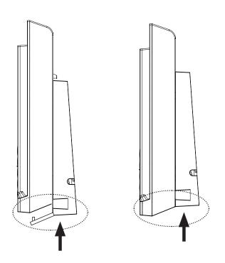
Connect the telephone as described in "Telephone base installation" on page 9, but connect the short telephone line cord instead. Place the cords in the associated cable ducts. 4. Mount the telephone base on the wall by positioning the eyelets on the telephone base and the mounting bracket against the mounting studs. Then slide the telephone base down on both mounting studs until it locks into place.
