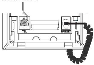
2. Align the grooves of the base stand with the telephone base. Slide the base stand up to secure it.
